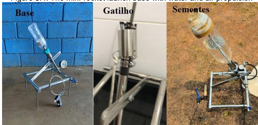
Figure 3.4. The mini-rocket launch base with water and air propulsion
