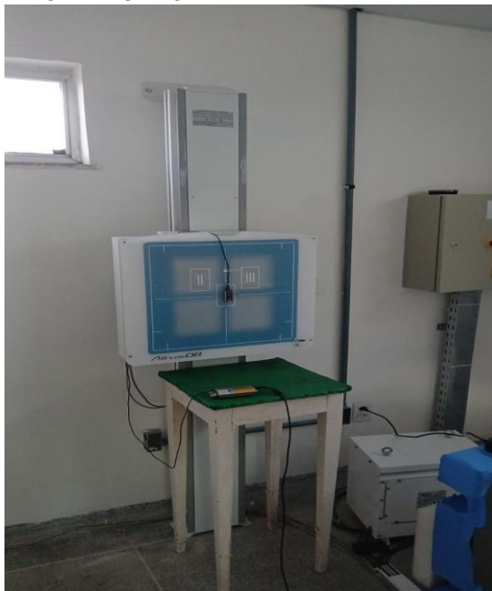
Figure 3 – Radcal® AccuGold® Solid State Sensor and Ionization Chamber
