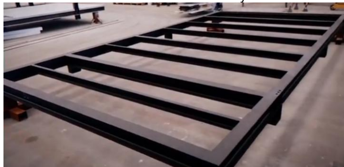
Figure 21 – Base of the module at the factory – metal floor chassis
