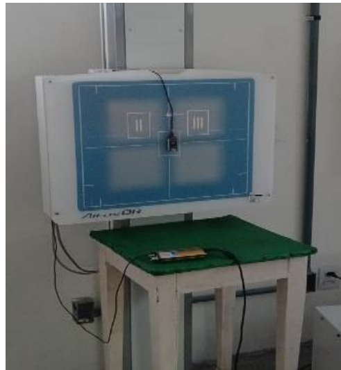
Figure 3 – Radcal® AccuGold® Solid State Sensor and Ionization Chamber
